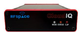
The Cloud-IQ is a Software Defined Radio (SDR) receiver with ethernet connection for the frequency range from 9 kHz to 56 MHz. The US-based manufacturer RFspace is well known for his excellent SDR receivers, the Cloud-IQ is the result of experiences collected with prvious products.
