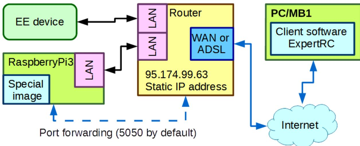
Using this way, ColibriDDC and RPi3 should automatically get IP addresses from a router (SunSDR2 PRO has a static IP). You need to set port forwarding (5050 by default for ExpertRS and 80 if you want to use the device via WEB-client) in the router to the RPi3 IP address, the example is in the Paragraph #3. Now you can use your device remotely.
