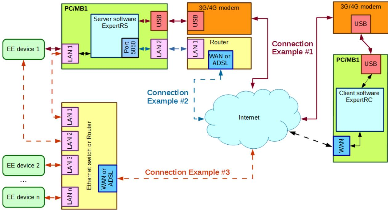
Figure 2 - Detailed remote control schematics
