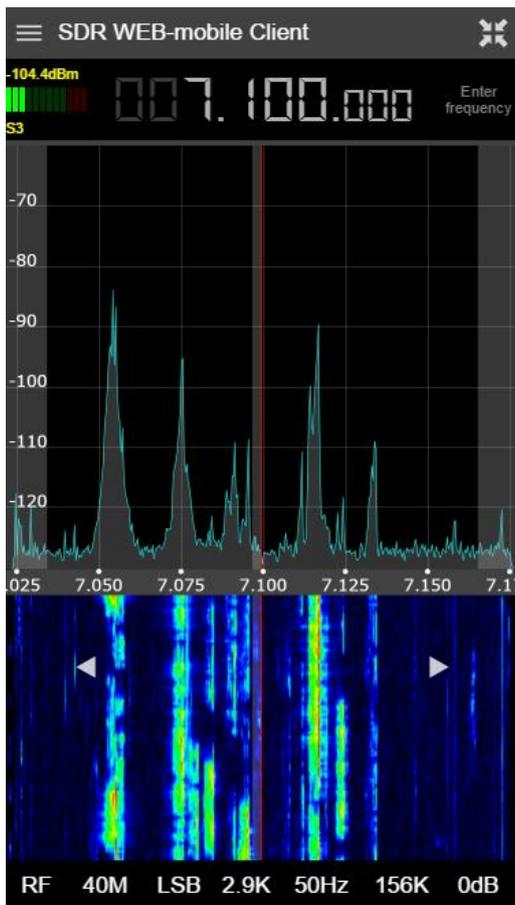
The main difference with the PC version is the tuning method. You can enter the required frequency or you may use touch screen to tune it, then browse left/right using the arrows on the waterfall with the set Step to perform fine tuning. By dragging the left vertical bar, you can change the noise floor level and by dragging the right vertical bar, you can change the ratio of the spectrum.
