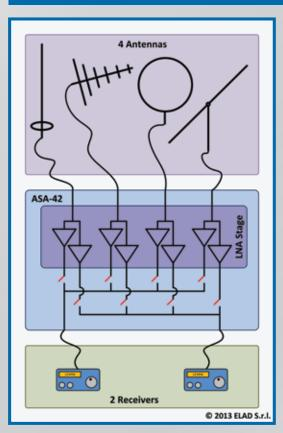
The **ASA42** Splitter Amplifier has been designed to split the signal received from four antennas to up to two different receivers at the same time.
