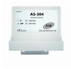
The antenna switch AS-304 is an electrically operated switch for four antennas. The unit is built into a weaherproof housing with mast mount. The switch is equipped with highly loadable power relays. In the result this High Frequency Switch is recommendale for a variety of tasks due to its big frequency range and the high power capacity. The according antenna is selected by simply putting the operating voltage of 12 V DC to one of the three Plus-PINs of the DIN-connector.
